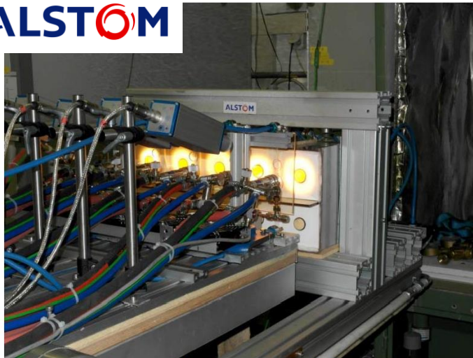
Figure 1. Picture of the burner rig test showing the two rows of 5 samples each
